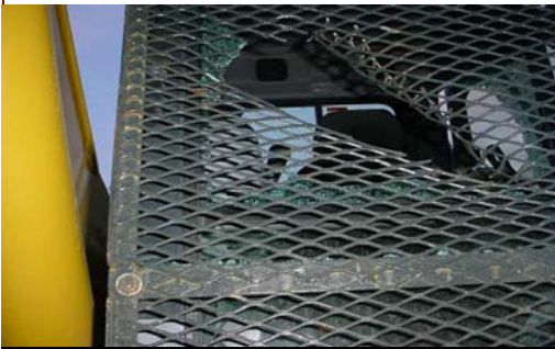
Metal Screen Guard & Window Penetrated by 19" Long Pipe
