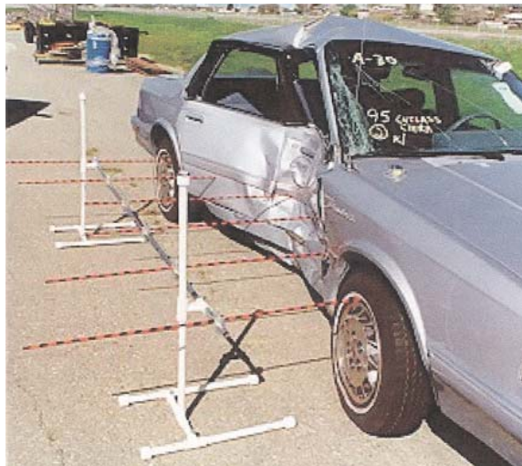
Measurement of crush depth: courtesy of Atlanta Engineering Services (I-ENG-A® Member Atlanta), Elvin Aycock, PE
